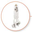
Made from Stainless Steel 316 grade to provide high corrosion resistance. Provides swageless termination to the cable. Fits 08mm diameter cable. Fixed at one end of the lifeline.
